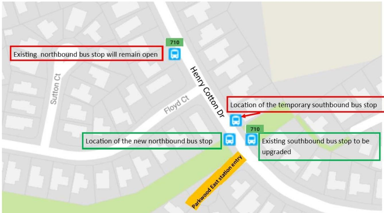
**Construction near the Parkwood East station entrance will continue with the installation of a new bus stop and the upgrade of an existing bus stop at the front of the new station on Henry Cotton Drive. This work will start the week commencing Monday 13 November 2017 and is expected to take up to five weeks to complete, weather and construction conditions permitting.**
